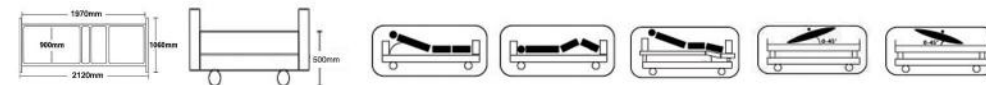
Bed size 床面尺寸 2100x1060 MM Bed surface height 床面高度 500MM Back rest lifting 背部升降 0-80° Leg rest lifting 腿部升降 0-25° Leg rest dropping 落腿 -65° -0° Left & right turn over 左右翻身 0° -45°
